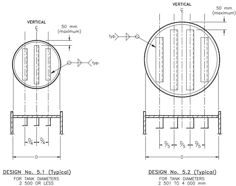
CONTINUOUS WELD SIZE:  $(t_h)/2$  but not less than 3 mm.
